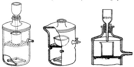
are to be filtered the shelf is removed and a large beaker inserted; or the jar itself may be used very conveniently, the three small protrusions interfering but little in washing, and the pouring lip facilitating the emptying of the jar.
